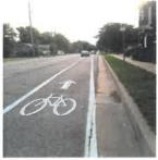
Bike lanes or additional roadway striping may be used to provide additional access to designated bicycle traffic on the roadway, or as a narrowing technique to better control for the speed of traffic.
