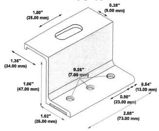
3 holes are provided for versatility. Some installations require only 2 fasteners. See the load table on the S-5! website and the installation instructions for more details.
