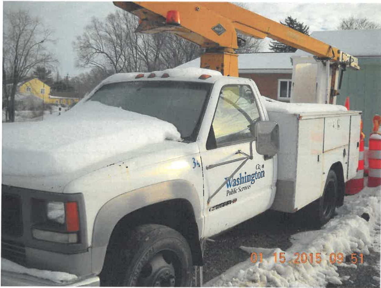
1994 GMC Sierra Bucket Truck with Versa lift Aerial (Current City Equipment)
