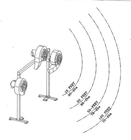
AMBIENT NOISE WITH AIR DRYER OFF: 70 dba.
