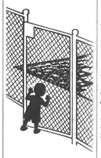
When the release mechanism of the self-latching device is less than 54 inches from the bottom of the gate, the release mechanism for the gate should be at least 3 inches below the top of the gate on the side facing the pool. Placing the release mechanism at this height prevents a young child from reaching over the top of a gate and releasing the latch.
